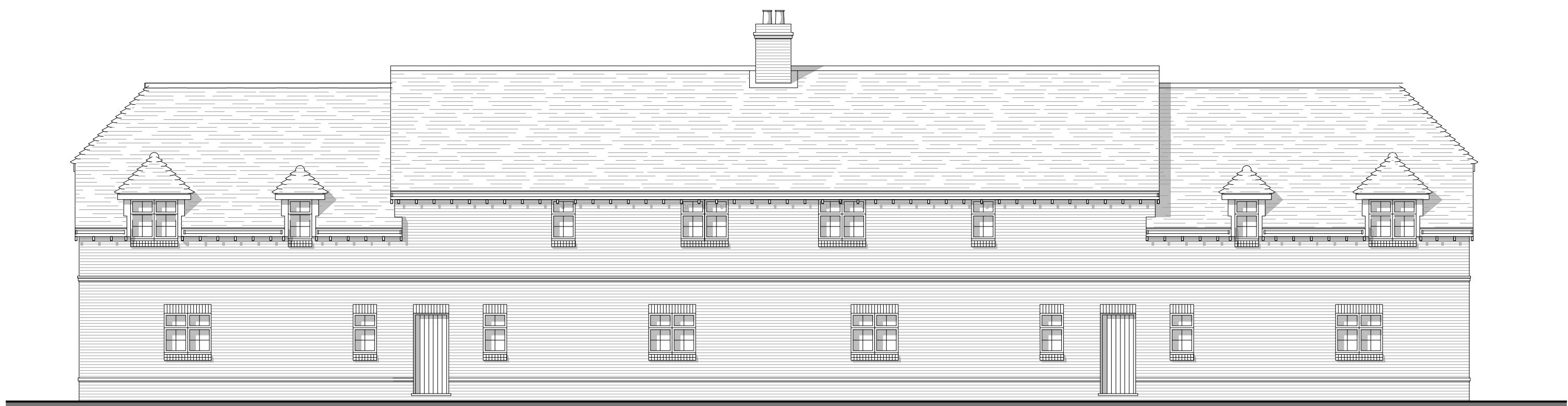
REAR ELEVATION NORTH NOTE ALL WINDOWS TO REAR ELEVATION TO BE OBSCURE GLAZED
